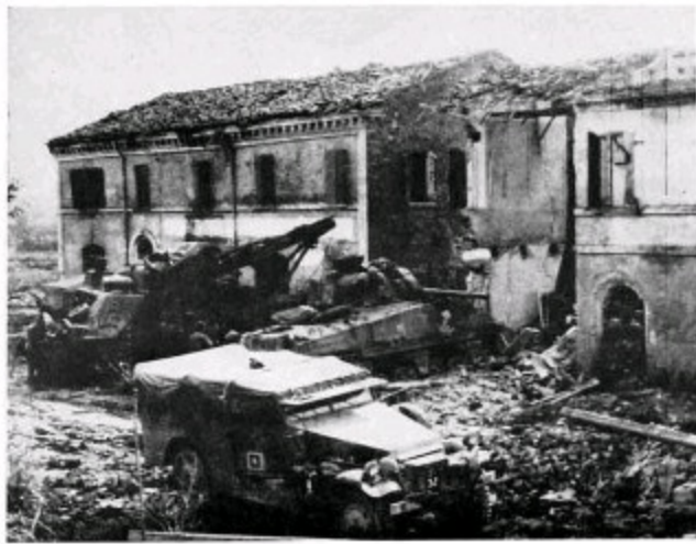
T2 recovery tank freeing a Sherman which broke its track when attempting to burst through this building. B Squadron's 'flying fitters' armoured car in the foreground
