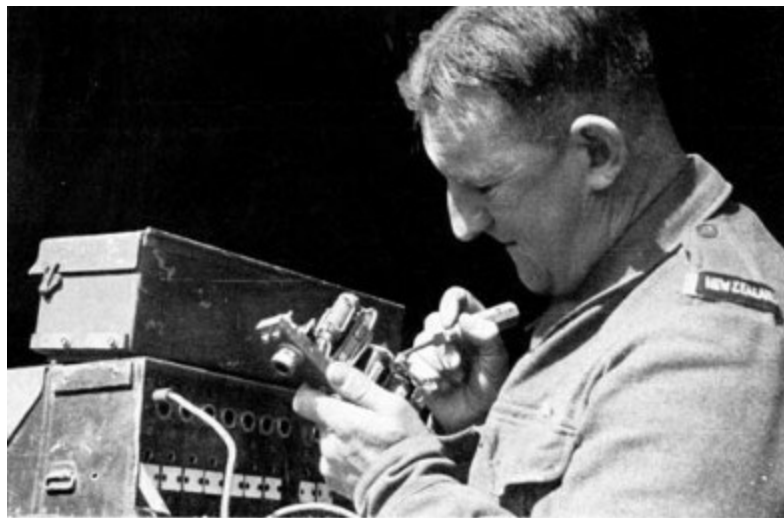
Adjusting an exchange relay at Cassino. A. B. Smith is the instrument mechanic
