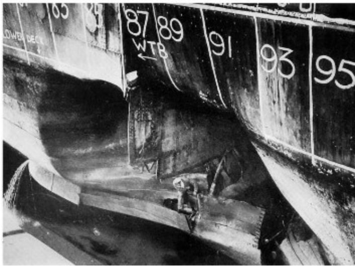
DAMAGE TO THE SIDE OF THE LEANDER
