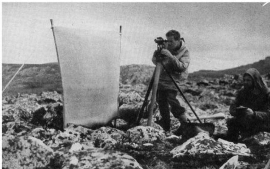
A surveyor takes observations. His theodolite is sheltered from the wind by a screen
