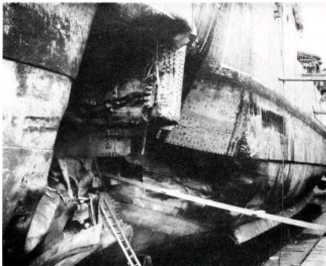
Leander in Calliope Dock, Auckland, showing torpedo damage
