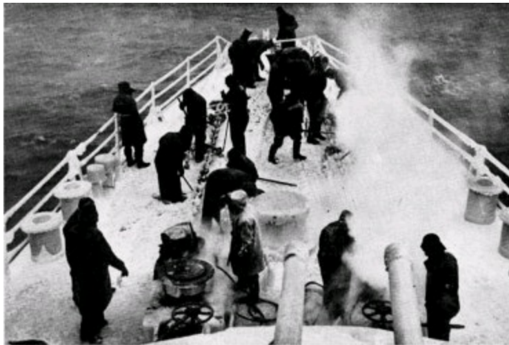
Steam jets clearing ice from anchor chains and windlass of a destroyer in a northern convoy
