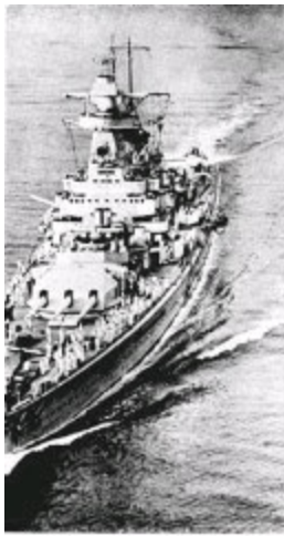
The Admiral Graf Spee , with six 11-inch guns in two triple turrets
