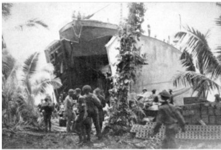
A LANDING SHIP (TANK) BEACHED AT MONO ISLAND Marsden matting helps unloading operations
